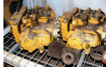
MAIN VALVE GROUP
