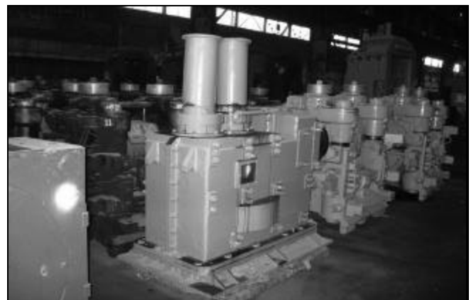
12" MUELLER NEUMANN 6-STAND FINISHING MILL
